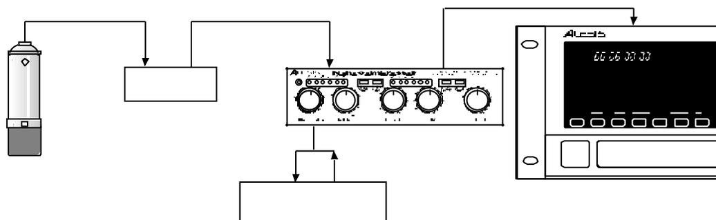
The trick is to set the EQ to cut all frequencies except for the sibilant range, between 3-6kHz. Then set the NanoCompressor like this:
