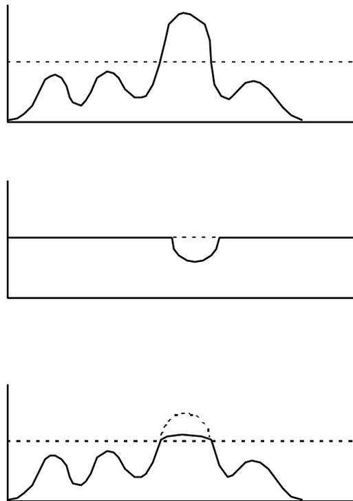
In the diagram above, Figure (a.) shows the input signal to the NanoCompressor. In this example the compressor Threshold is set for -10dB and the Ratio is set for 4:1. When the third peak of the input signal crosses the Threshold, the NanoCompressor starts to reduce the signal level, as shown in Figure (b.). Figure (c.) shows the output signal level, with the original signal shown with a dotted line.
